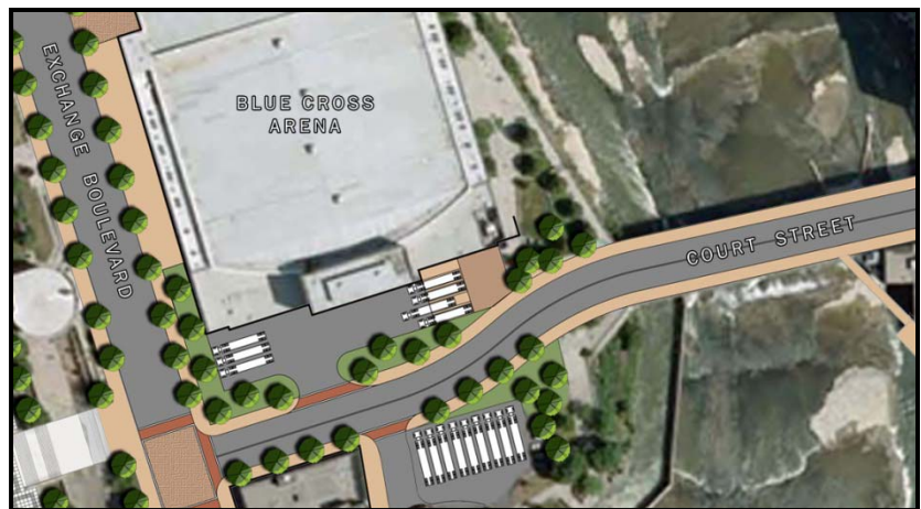
Realigning the western terminus of Court Street slightly to the south will provide designated space for truck staging and queuing preventing the need to close Court Street to through traffic during large events at the Blue Cross Arena
